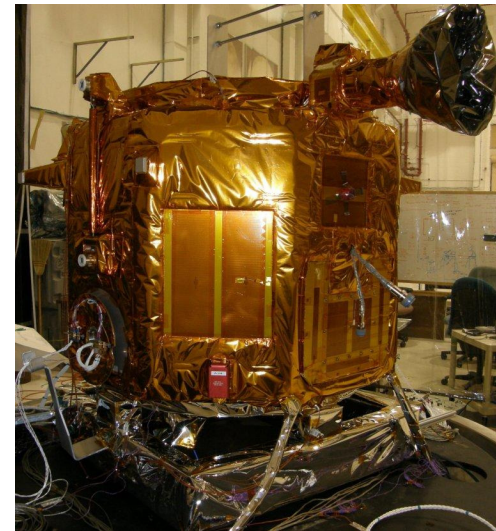
ORS phase III bus preparing for TVAC testing
